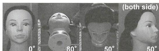
Fig.4 Functional limit of face tracking
